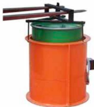
Top, bottom or side flanges may be used to attach handling equipment, if preferred to manual lifting. A range of dedicated products is available but many standard forms of handling device are suitable.
