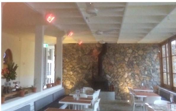
**Halogen infrared is the most efficient method of providing comfort heating to a closed in outdoor room.**
